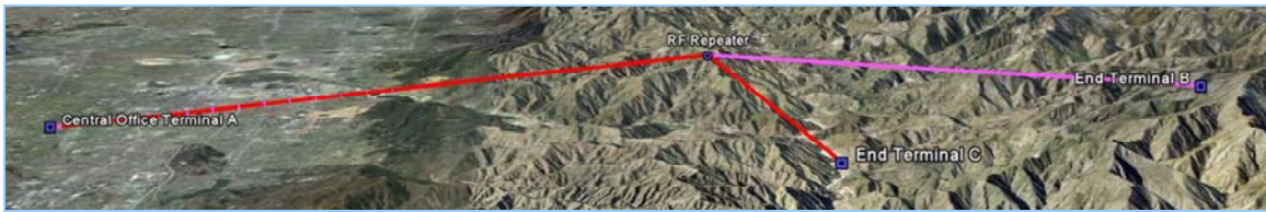
Figure 3 RF-11000 Y-Junction Repeater, 3-Hops
