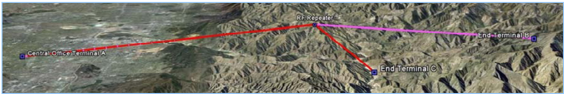
Figure 3 RF-6000EW Y-Junction Repeater, 3-Hops
