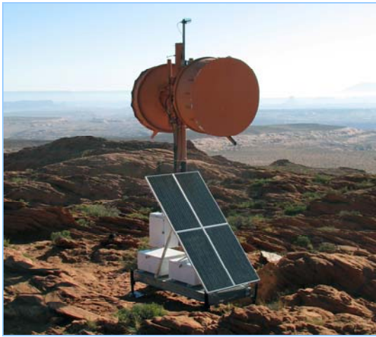
Figure 1 RF-6000E Solar Powered Repeater
