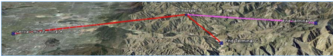
Figure 3 RF-6000E Y-Junction Repeater, 3-Hops
